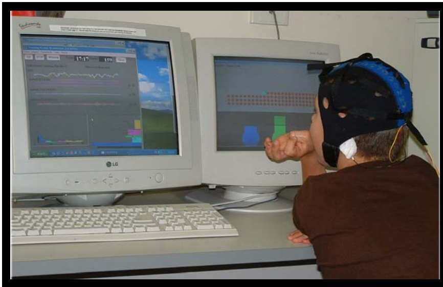
Photo 1: Student involved in a training session. Electrode cap ensures correct placement of electrode lead
